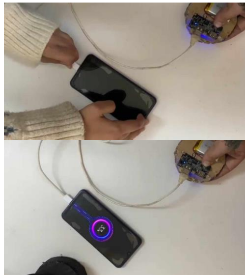
Figure 13: Using the back part of the unit prototype to recharge a mobile battery.
