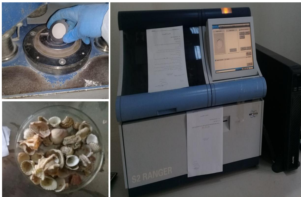
Figure 2: Analyzing shell samples, and preparing for XRF scanning with S2 Ranger 2008.
