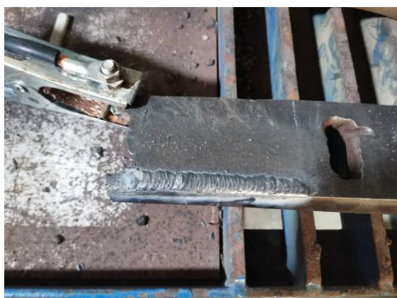
Figure 2a: Shows the Experimental Set up. 2b: The image shows a flat metallic specimen on which an electric arc welding bead has been deposited using a metal electrode.
