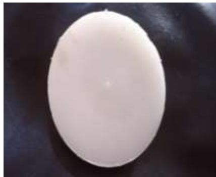
(c). Prepared HDPE sample.
