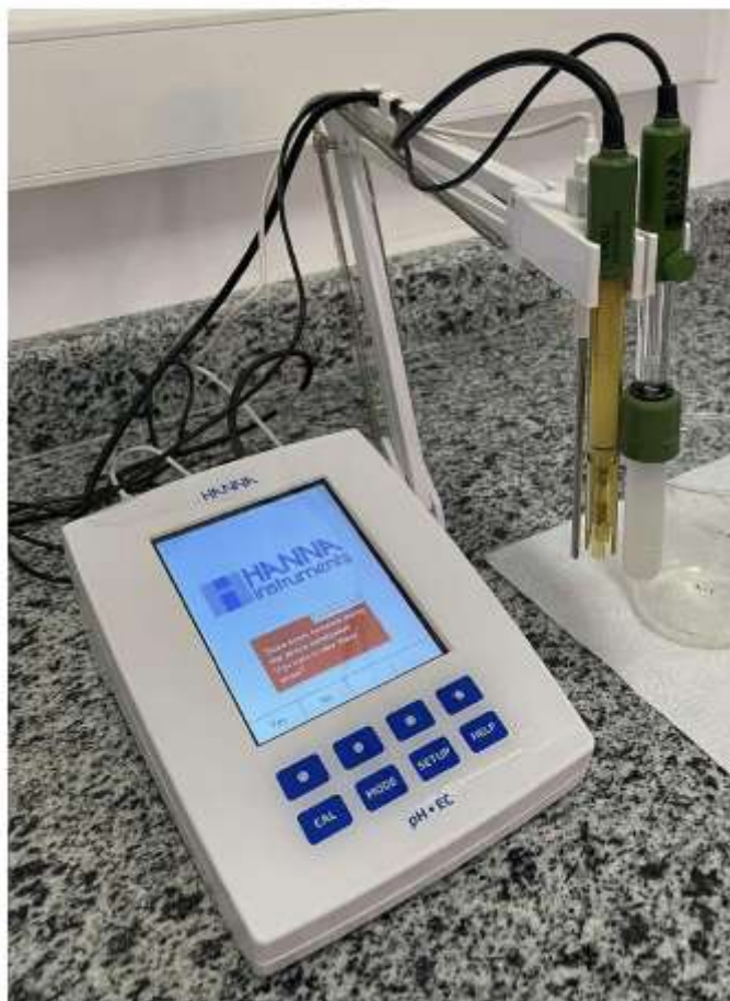
Figure (2) Device used to measure pH, electrical conductivity, and total dissolved salts.
