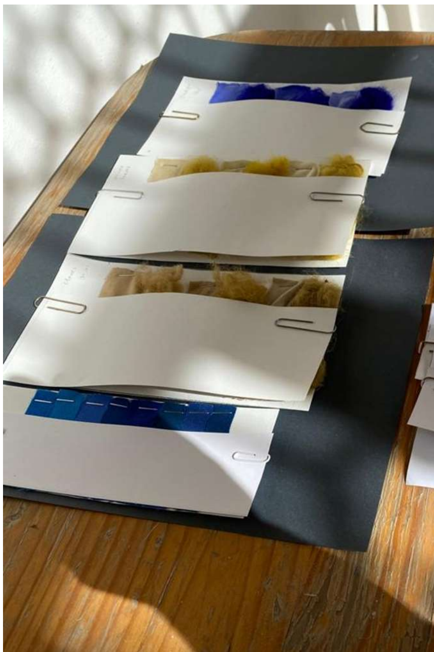
Figure (5) Exposing the experimental samples to daylight.
