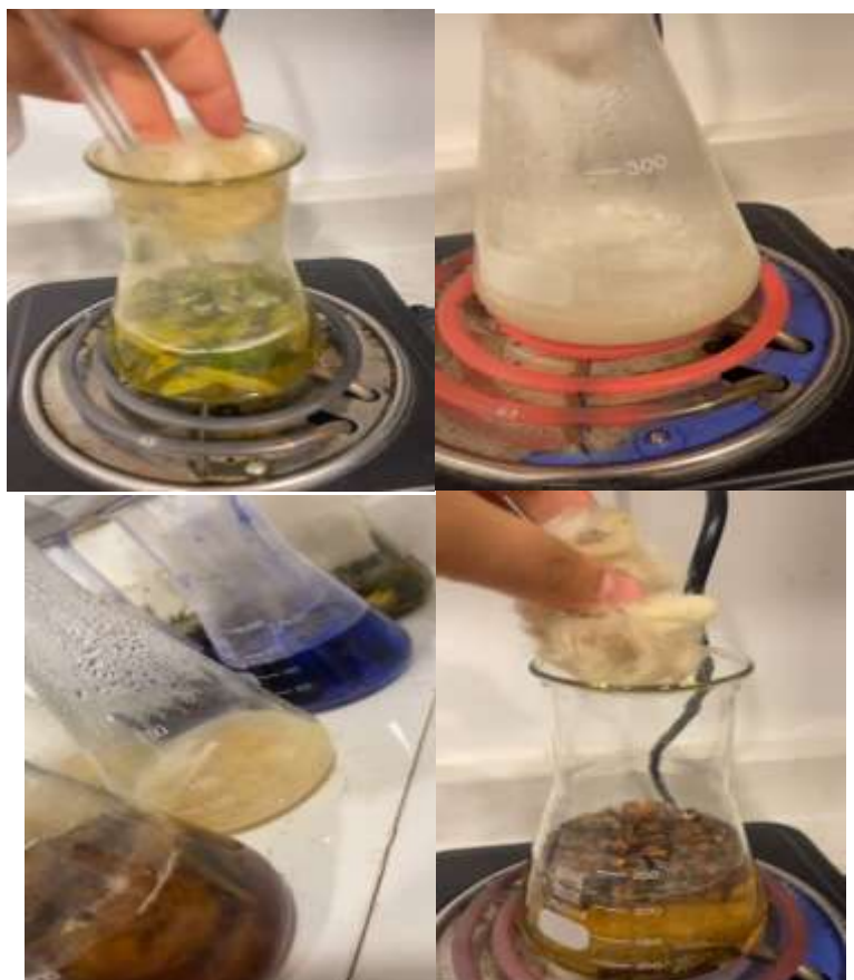
Figure ( 3 ) Fixing the experimental samples in the net and dyeing the experimental samples in dye solutions.
