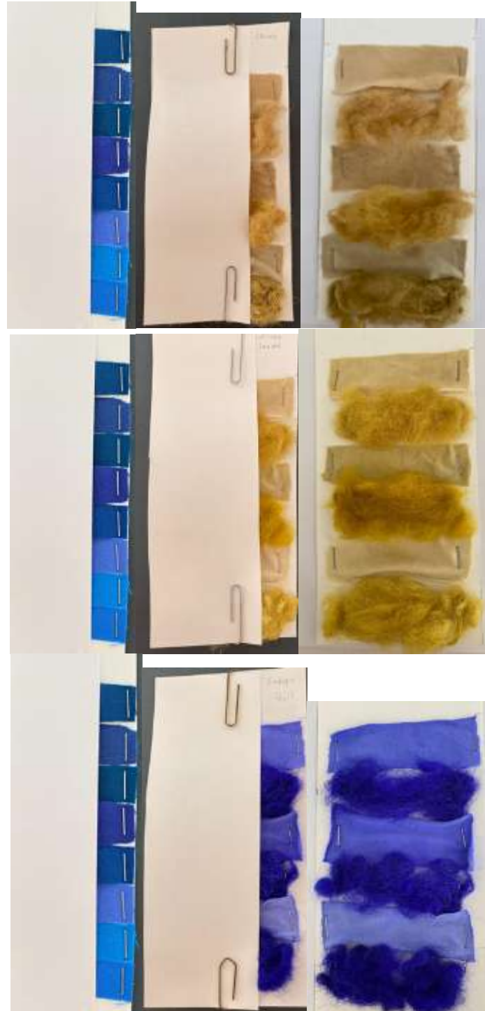
Figure (4) Preparation of wool and cotton blend samples for light testing, accompanied by the standard blue wool guide.
