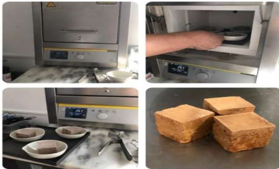
Figure 8: The Firing Apparatus and the Fired Sample .
