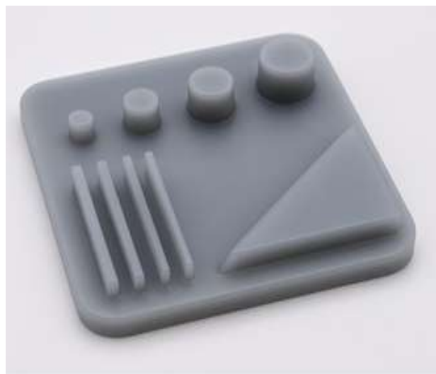
Figure 5. SLA-printed artifact showing fine thin walls and wedge transitions.
