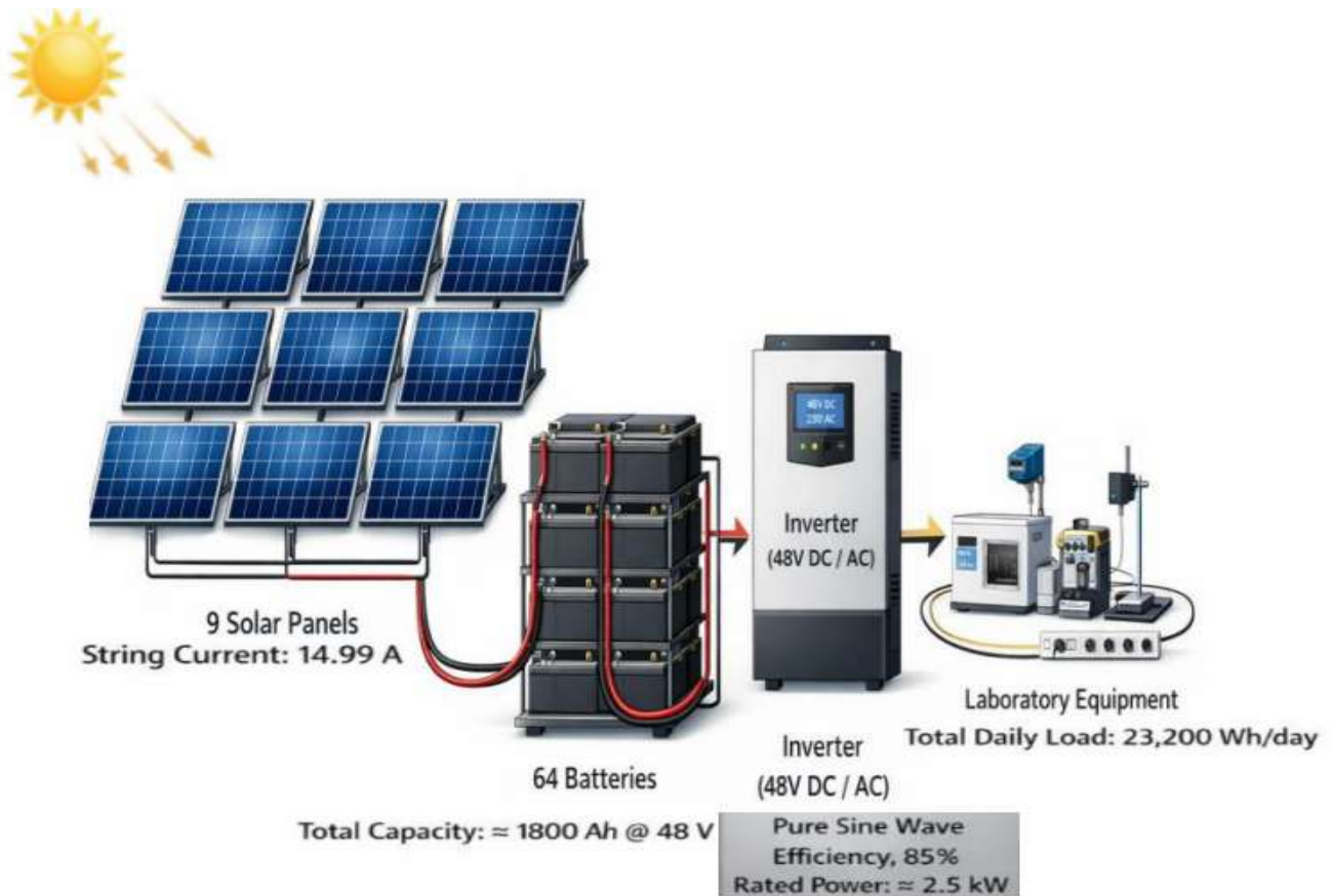
Figure 16: 3D schematic layout of the designed a photovoltaic system for the drilling fluids laboratory
