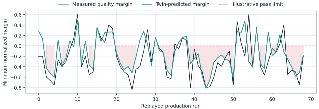
Figure 9 Replayed production sequence using measured and predicted quality margins.
