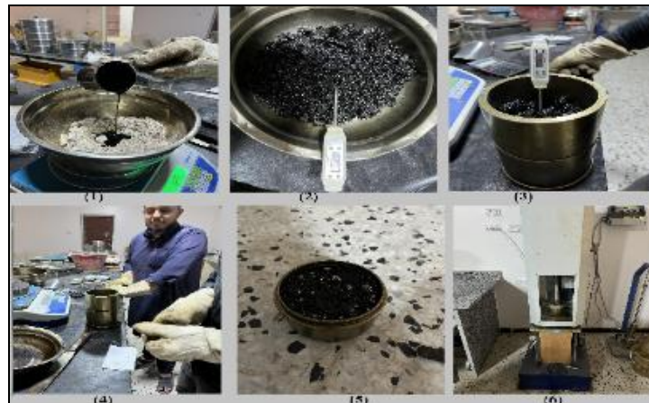
Figure 17: Show the main stages of Marshall stability test.
