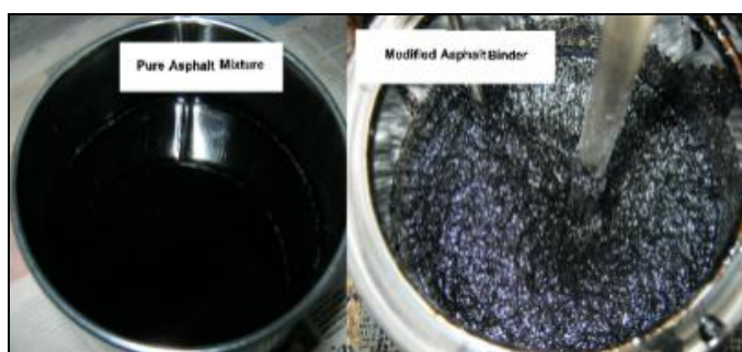
Figure 18: Represent pure and modified asphalt binders.
