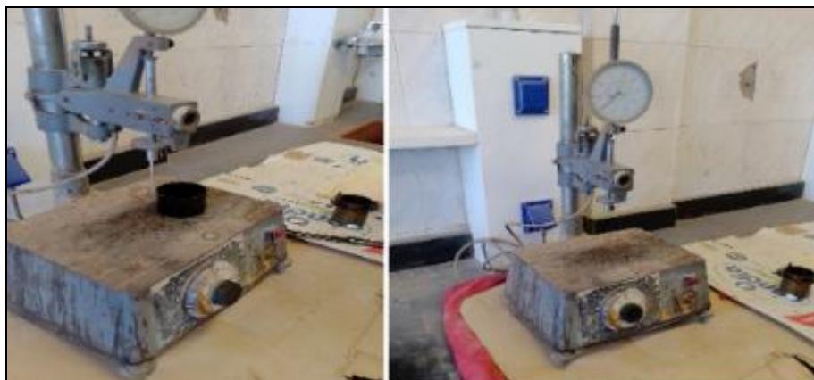
Figure 15: Asphalt penetration test.
