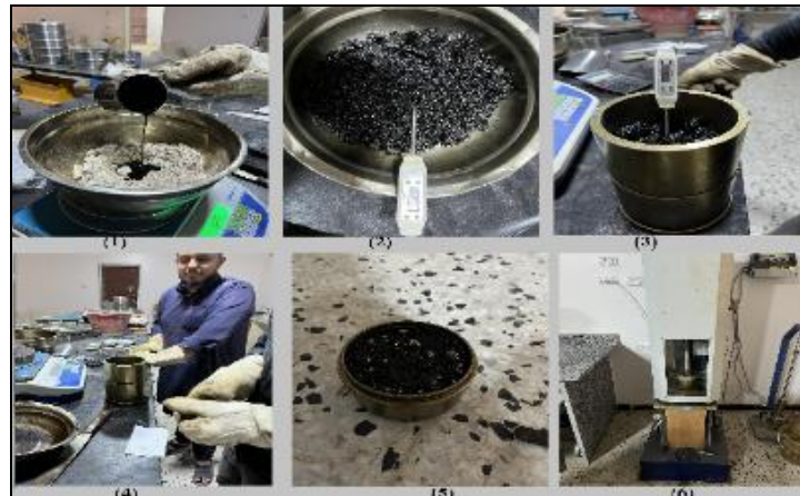
Figure 17: Show the main stages of Marshall stability test.
