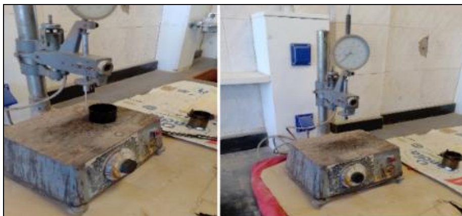
Figure 15: Asphalt penetration test.
