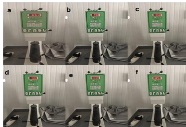
Figure 4. Representative Rockwell hardness tester readings for the investigated heat-treatment conditions: (a) As-Cast, (b) Annealed, (c) ST-Q, (d) T6-4h, (e) T6-8h, and (f) T6-12h.
