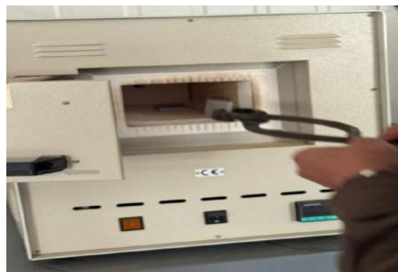
Figure. 1. Electric box/muffle furnace used for the heat treatment of the EN AC-43000-F specimens.
