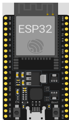
Figure1: ESP3 Pinout and Board Layout (Espressif systems,2026)
