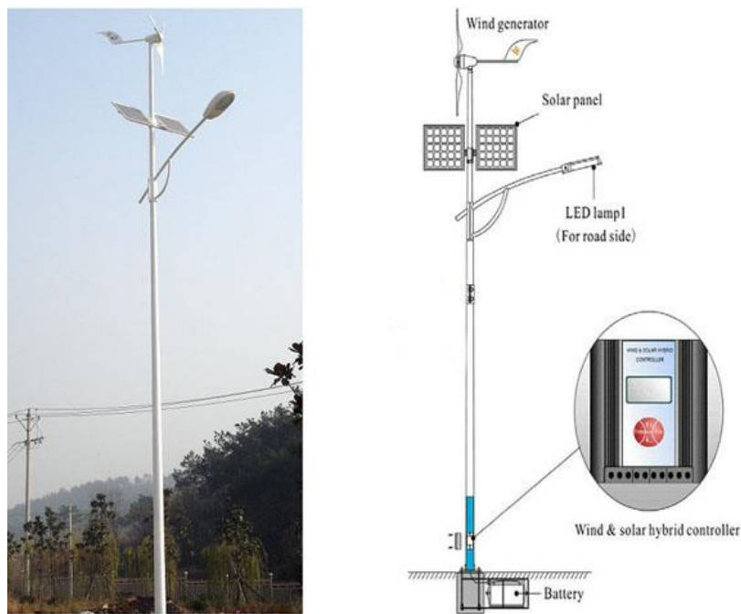
Figure 11 Hybrid solar/wind street lighting system [11].
