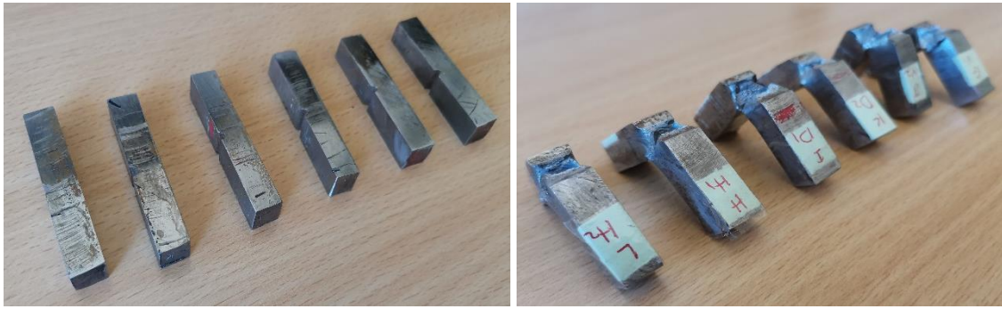
Figure 10. Fractured samples after impact tests
