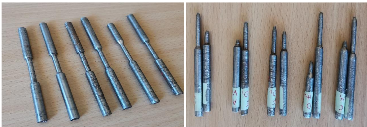
Figure 9. Fractured samples after tension tests
