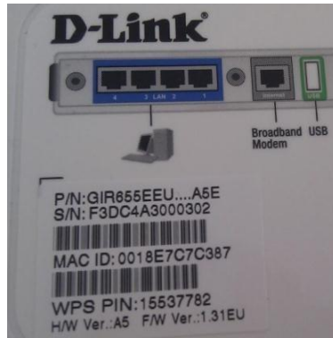
Figure 10: Label with WPS PIN on the back of a D-Link router [18]
