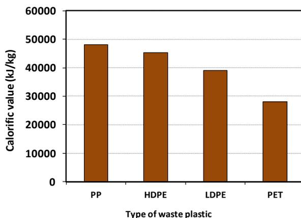
**Figure 5:** Comparison of calorific value for the produced oil.
