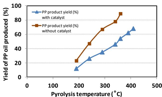
**Figure 6:** The effect of pyrolysis temperature on PP liquid product with and without catalyst.
