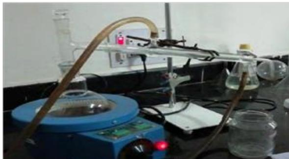
**Figure 2:** The distillation process of plastic oil.
