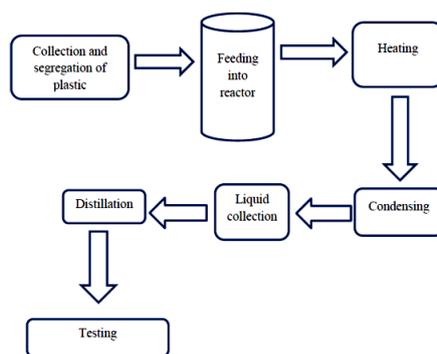
**Figure 1:** The main steps for pyrolysis process of waste plastics
