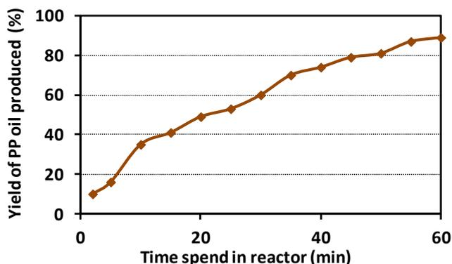
**Figure 7:** The yield of produced oil from waste PP against time spent in the reactor.
