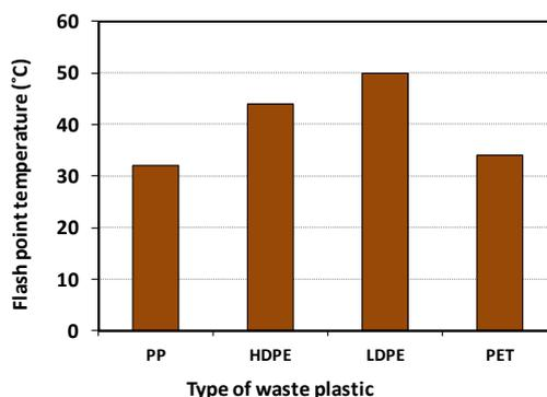
**Figure 3:** Comparison of flash point for the produced oil.
