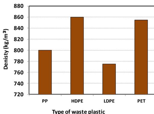
**Figure 4:** Comparison of densities for the produced oil
