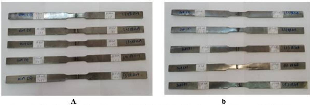
Figure: 3 (a): Specimens Tensile test with ER2209, (b): Specimens Tensile test with ER308
