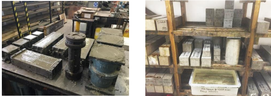
Figure 2: Casting and curing of specimens.
