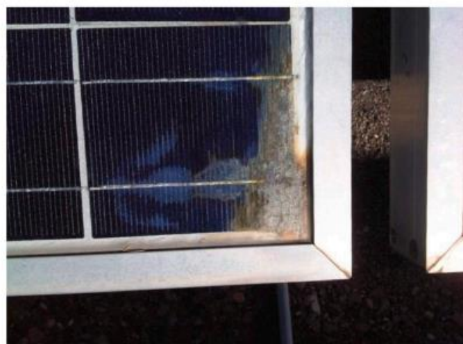
Figure 2: A typical moisture ingresses PV module showing signs of corroded metal grids, delamination and discoloration of encapsulants.
