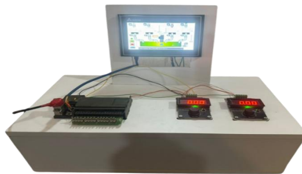
Figure 10: The Automated Concrete Machine Using PLC and HMI Control System
