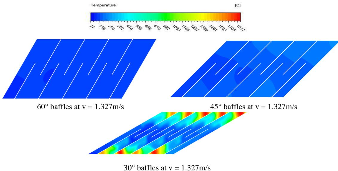
**Figure 5** Temperature contour of the absorber plate via different short baffle angles at  $1.327\text{m/s}$
