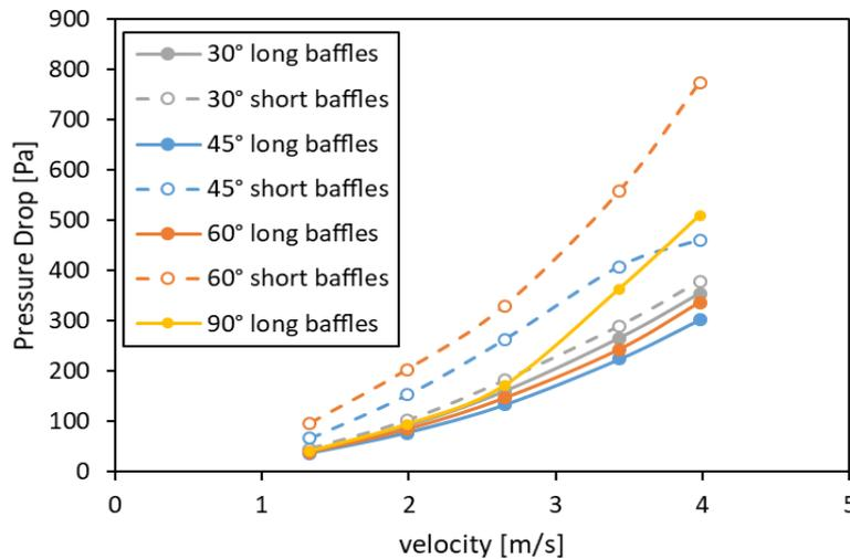
**Figure 6** Pressure drop at different inlet velocities for long and short baffles.
