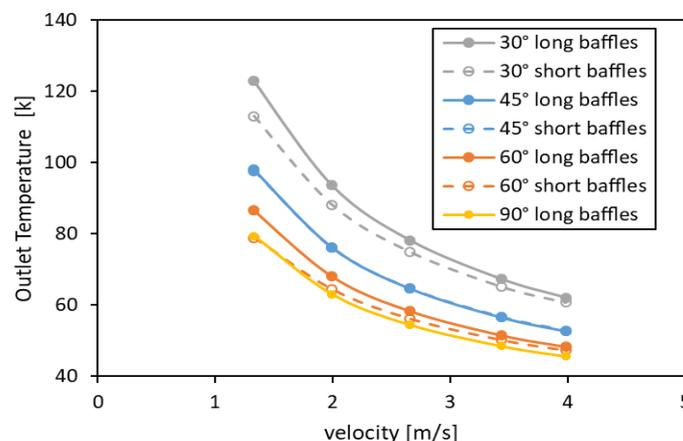
**Figure 3.** Air outlet temperature at different inlet velocities for long and short baffles.
