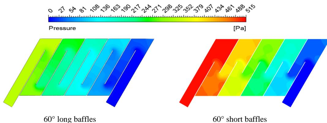
**Figure 7** Pressure distribution at 3.983m/s for long and short baffles
