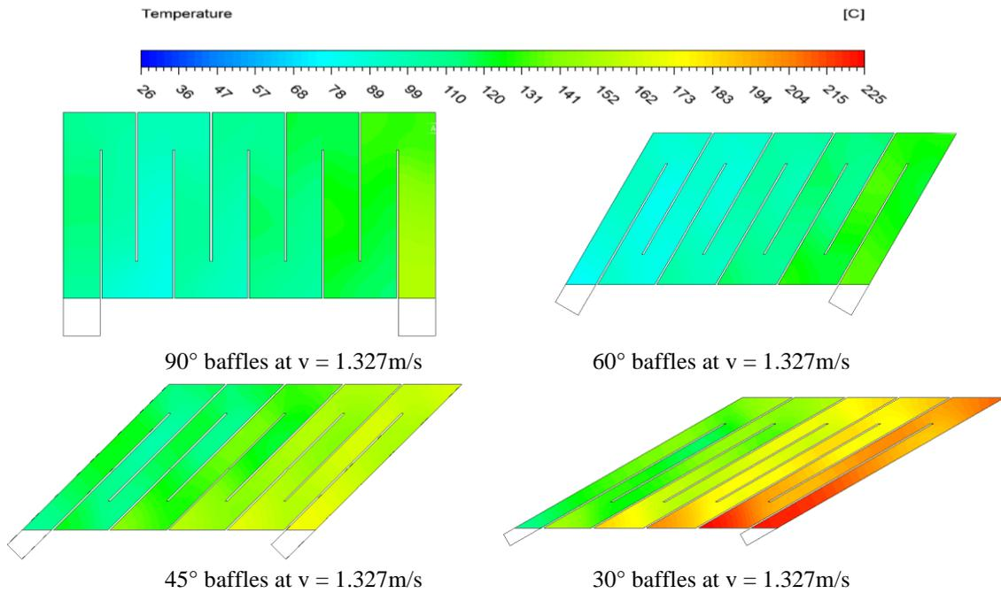
**Figure 4** Temperature contour of the absorber plate via different long baffle angles at  $1.327\text{m/s}$
