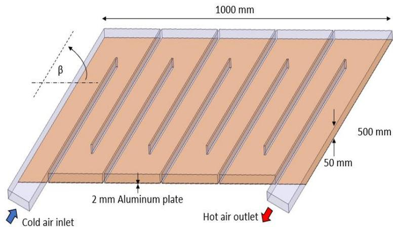
**Figure 1.** Schematic view of the air duct with the plate.
