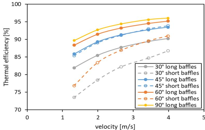
**Figure 8** Thermal efficiency at different inlet velocities for long and short baffles.
