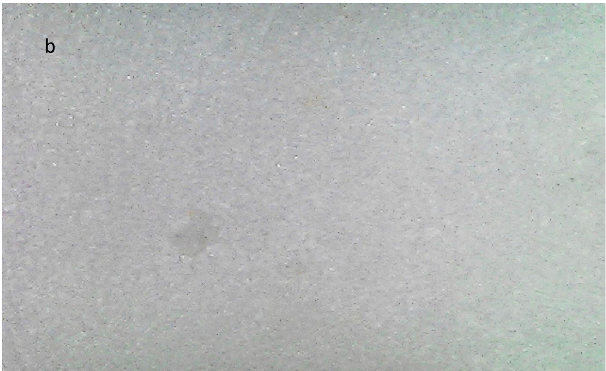
Figure 4 Microstructure of the surface of (a) pre-sintered and (b) sintered HT4 zirconia at magnification of 150 ×
