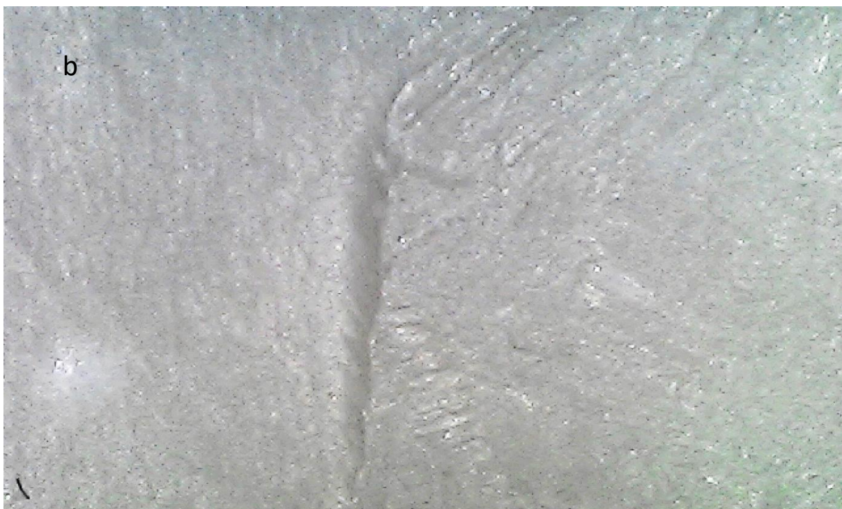
Figure 5 Microstructure of the surface of (a) pre-sintered and (b) sintered A214 zirconia at magnification of 150 ×
