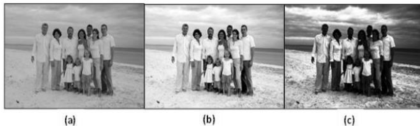
Figure 2: Pre-processing an input image: (a) Convert the image to grayscale, (b) Normalize the image, and (c) Enhance the contrast.
