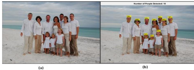
Figure 10: The final result of counting people: (a) Original image and (b) Using FrontalFaceCART.
