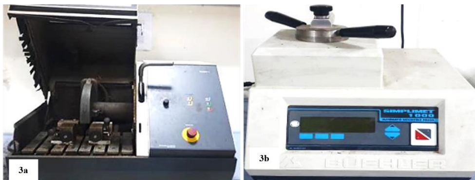
Figures 3a and b: The Cutting Machine and Molding Device Respectively.
