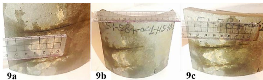
Figure 9a, b and c: The External Shape of the Specimen and the Approximate Length of the Notch after Cutting.
