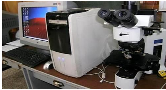
Figure 5: The Olympus Light Microscope and their Accessories.
