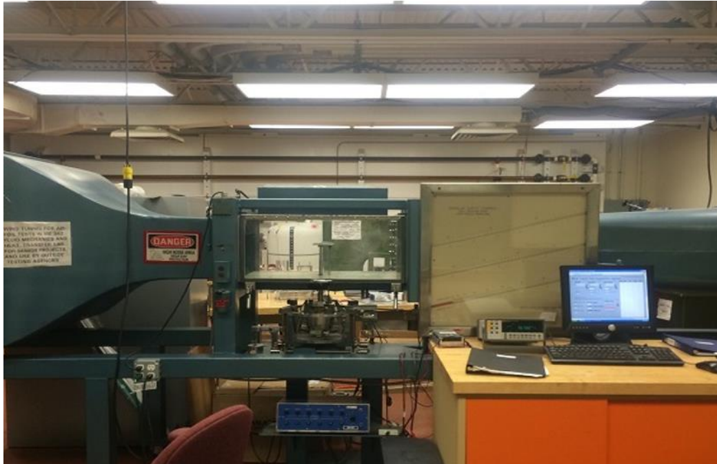
Figure 1 : A low-speed wind tunnel at the University of Hartford.
